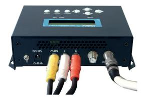
**4.** Connect the power to the wall outlet with the power adapter.
